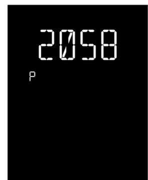
The offset value of the **pressure sensor** is displayed approximately two seconds later.
